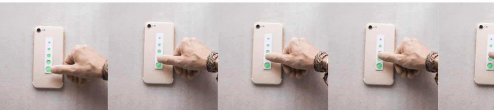
Figure 20. Use and interaction with the prototype of the saving-kit: a phone case that would allow saving by sliding up one's finger
