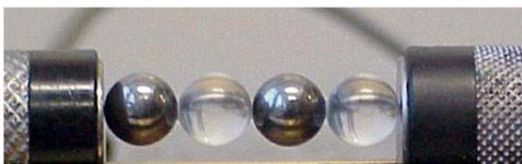
FIGURE 2.34: Sample of the phononic crystal studied in reference [28], also showing the experimental set-up
