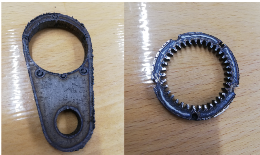
Figure 5.2: Laser cut housing and gear. The thick material causes the cut surface to be very rough and thereby inaccurate.
