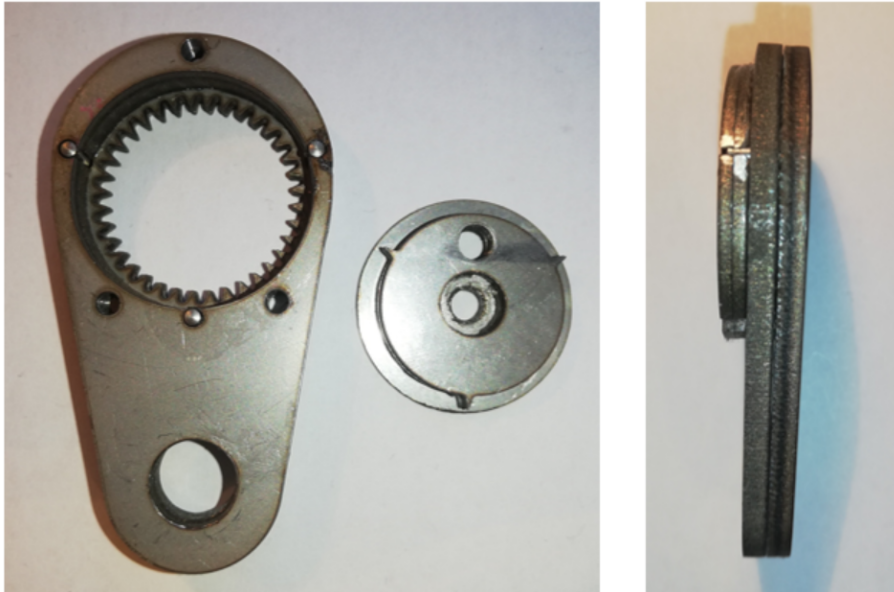
Figure 5.3: Laser cut housing and gear using thin sheets of steel. The gear parts are build up from 2 mm steel. The remainder of the housing is made of 3 mm steel sheets. The Housing is held together using dowel pins.
