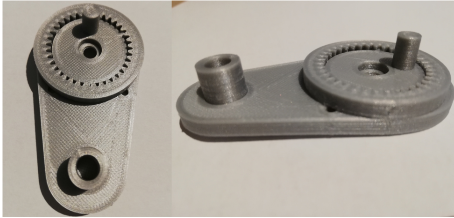
Figure 5.1: PLA print of the gear and housing of the prototype. As can be seen on the right, the gear is not flush with the housing. This is due to limited capabilities of the 3D-printer.
