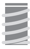
Use a conductive material around the bin and cool this down with water.
