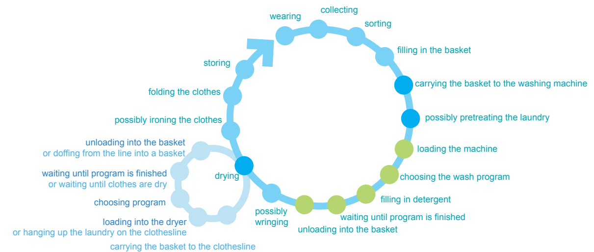
Fig. 3: General washing cycle with a drying sub-cycle, developed by the author after seven years of washing process user observations and interviews. The green steps mark the tasks, which involve the washing machine; the darker blue steps indicate steps, which might involve the washing machine. The pale blue sub-cycle illustrates the drying cycle, which comprises two possibilities: using a dryer or hanging up the laundry on a clothesline.
