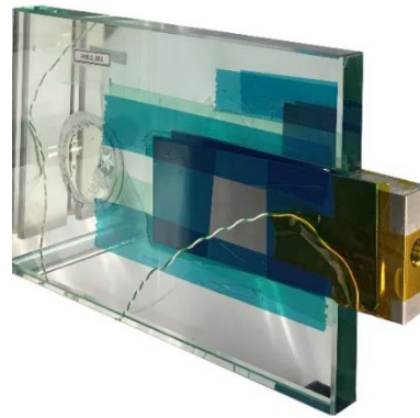
Fig. 2 Edge-laminated connection during fabrication process
