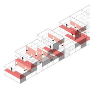
4. Execution of "blocks" - transformation of former apartments into new modules by punctures
