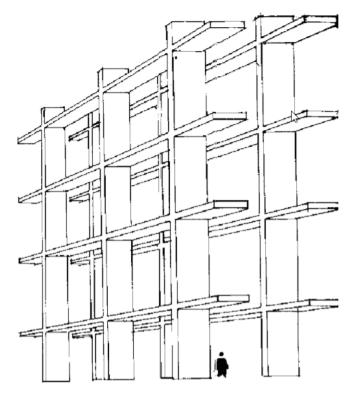
Figure 13 Separation of supports and infills, John Habraken. Drawing present the same principle as the ERA construction.
