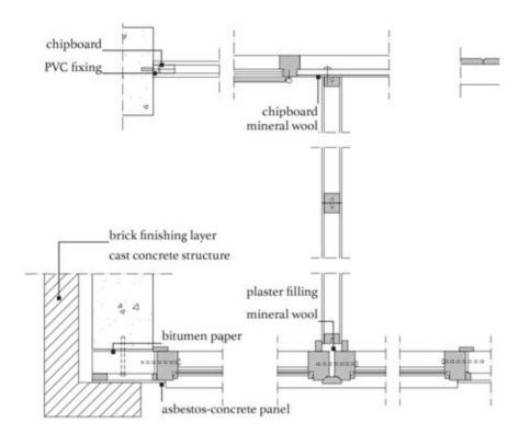
Figure 14 Details of construction, facade and interior walls connection. Here, in detail, the separation of the load-bearing structure and skin-elements such as façade or brick finishing layer is visible.
