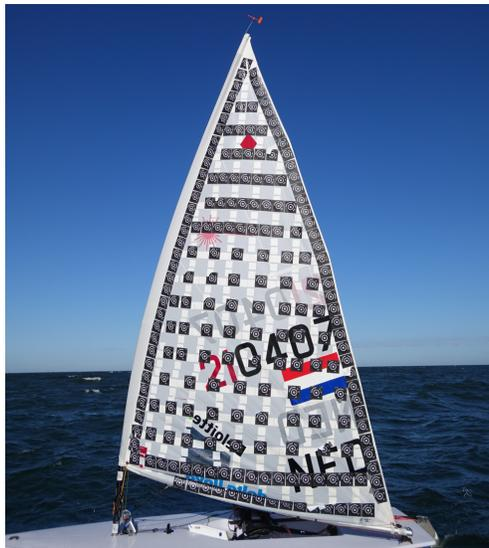
Figure 22: An image from which a sail measurement was generated by the Sailing Innovation Centre in collaboration with GeoDelta.
