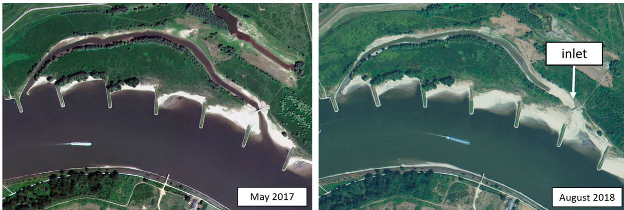
Figure 4. The side channel Klompenwaard during regular (left) and low-flow conditions (right). Due to low discharges the upstream inlet becomes dry and no inflow of the side channel takes place. Satellite images obtained from Netherlands Space Office.
