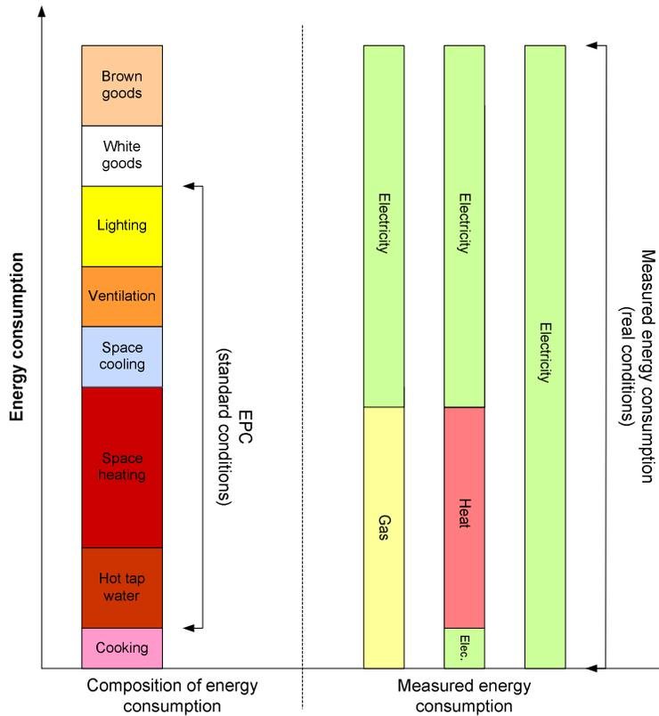
Figure 1: Build-up of the EPC and relationship with measured energy consumption.
