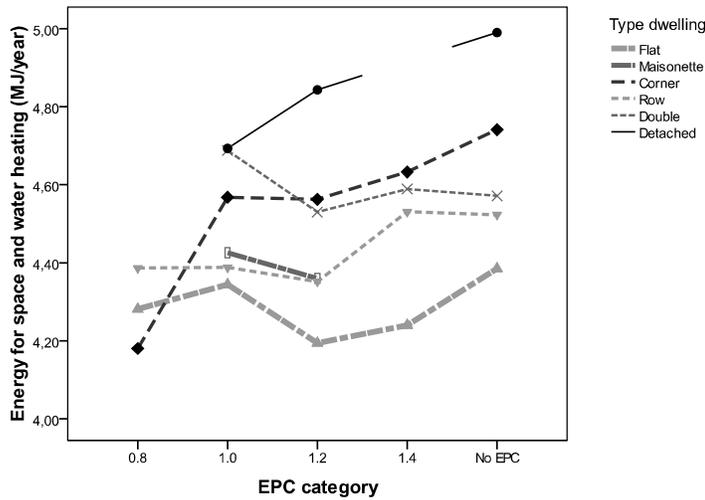
Figure 2: Energy used (mean LOG) per dwelling type and EPC level. For reasons of clarity, the 95% confidence interval is not plotted.
