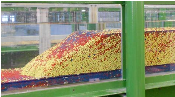
Figure 1. Flume experiment of a Gilbert delta using three well-sorted size fractions (fine blue, medium red, coarse yellow).
