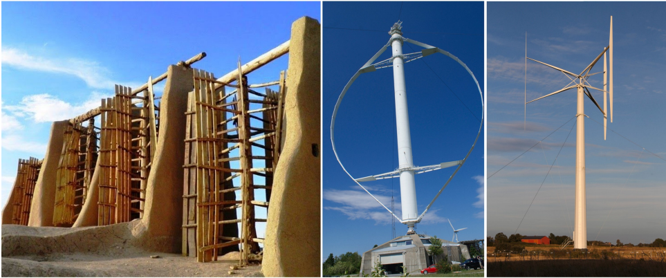
Figure 1.1: Left: Persian vertical axis windmills. Image from https://www.amusingplanet.com/2014/07/the-ancient-windmills-of-nashtifan.html . Center and Right: Modern \Phi -type and H-type VAWTs. Photos by Erik Möllerström (Möllerström et al., 2019).
