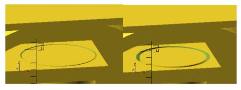
Figure 46. Effect of nozzle size to the clearance (left = 0.1 mm nozzle size, right = 0.4 mm nozzle size)
