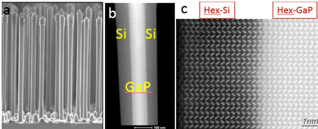
**Fig. 1:** Transfer of the crystal structure from a wurtzite GaP core wire into a Hex-Si shell. (a) SEM image of GaP/Si core/shell NWs, (b) TEM image of a Hex-GaP/Si core/shell NW, (c) High-resolution TEM image of GaP/Si interface confirming the hexagonal Si crystal structure.<sup>4</sup>
