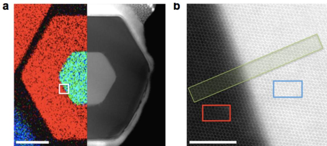
**Fig. 2 :** (a) cross sectional TEM image of a hexagonal GaP/Si core/shell nanowire illustrating the conformal epitaxial growth, (b) High-resolution TEM image of the GaP/Si interface substantiating the defect-free hexagonal Si crystal structure.<sup>4</sup>
