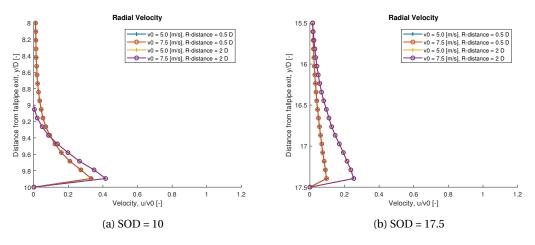
Figure 7.3: Normalized radial velocities for different input velocities and radial location
