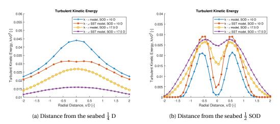
Figure 7.9: Turbulent kinetic energy for different turbulence models and location in the flow field
