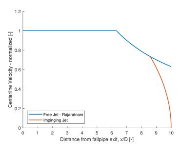
Figure 5.3: Normalized centerline velocity impinging jet region (large SOD)
