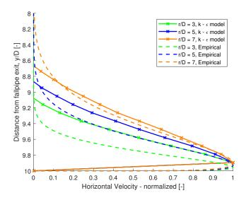
Figure 7.12: Normalized horizontal velocity comparison for the wall jet region, SOD = 10,  $k - \varepsilon$  model
