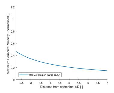
Figure 5.5: Normalized maximum horizontal velocity wall jet region (large SOD)
