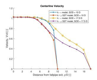
Figure 7.5: Normalized centerline velocities for different turbulence models and SOD
