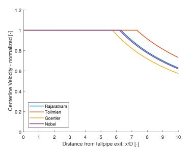
Figure 5.2: Normalized centerline velocity for the free jet region
