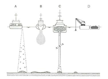
Figure 2.2: A) Side-stone dumping vessel, B) Split hopper barge, C) Fallpipe vessel, D) Dragline [Kevelam]
