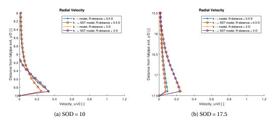
Figure 7.6: Normalized radial velocities for different turbulence models and radial location
