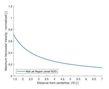
Figure 5.7: Normalized maximum horizontal velocity wall jet region (small SOD)
