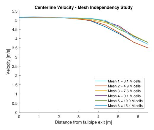
Figure D.1: Centerline Velocity - Mesh Independency Study
