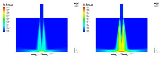
(a) Contour plot TKE for  $k - \varepsilon$  turbulence model (b) Contour plot
