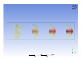
Figure 7.1: Velocity profile development fallpipe length section of  $4 \cdot D$
