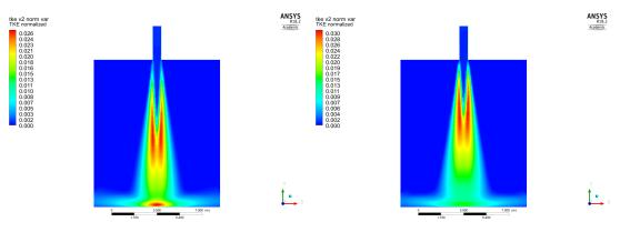
(a) Contour plot TKE for  $k - \varepsilon$  turbulence model
