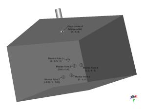
Figure D.5: Locations of the Monitor Points in the Simulation Domain
