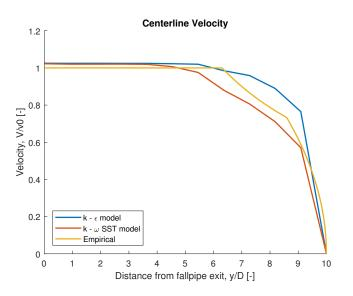
Figure 7.11: Normalized centerline velocity comparison for the impinging jet
