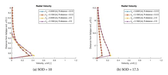
Figure 7.4: Normalized radial velocities for different  $k_s$  values and radial location
