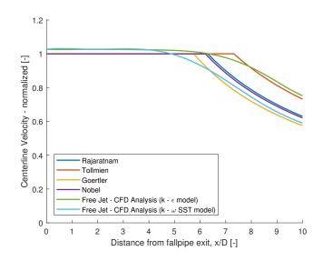
Figure 7.10: Normalized centerline velocity comparison for the free jet region
