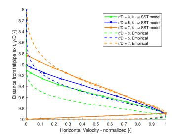
Figure 7.13: Normalized horizontal velocity comparison for the wall jet region, SOD = 10,  $k - \omega SST$  model
