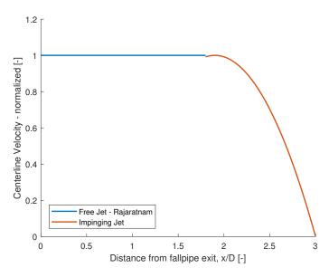
Figure 5.4: Normalized centerline velocity impinging jet region (small SOD)
