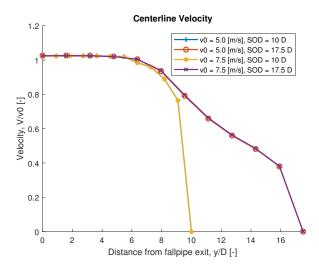
Figure 7.2: Normalized centerline velocities for different input velocities and SOD
