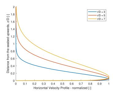
Figure 5.6: Normalized maximum horizontal velocity profile wall jet region (large SOD)
