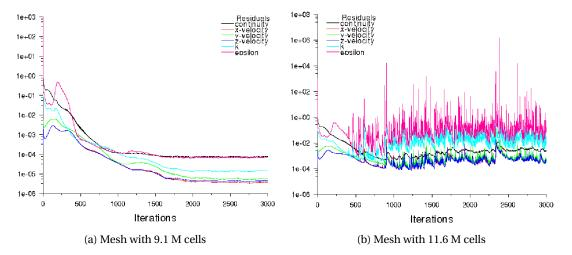
Figure D.4: Returning oscillating residuals for mesh refinement
