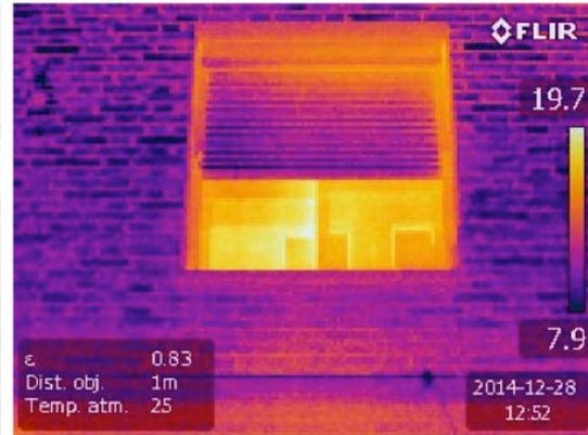
Fig 6: Outdoor infrared image. Non-renovated building.
