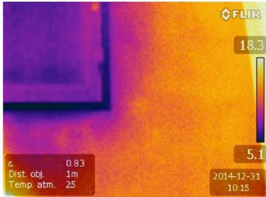
Fig 7: Indoor infrared image. Non-renovated building
