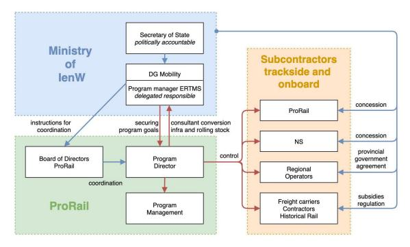
Figure 8: Dutch governance model for the ERTMS implementation. This is a translated model in the ERTMS implementation plan (Programma ERTMS, 2019).
