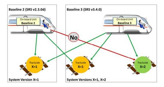
*Figure 5: Compatibility between on-board compliant with a specific baseline and tracksides operating with specific system version (UNISIG, 2014).*
