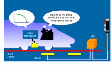
Figure 27: ERTMS/ECTS application level 1 without infill (ERTMS, 2020)
