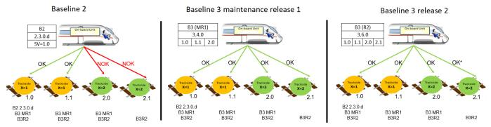
Figure 6: compatibility between SVs of on-board and trackside equipment. Edited image from Arenas (2015).
