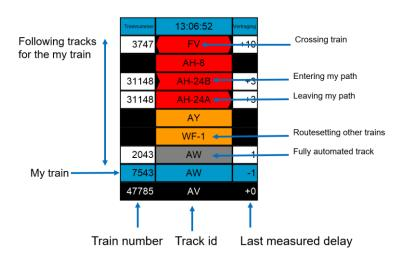
Figure 21: GUI (Graphical User Interface) by ProRail of RouteLint. Edited figure from van Luipen (2019).
