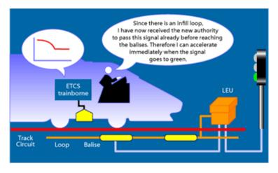
Figure 28: ERTMS/ECTS application level 1 with infill (ERTMS, 2020)
