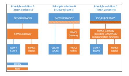
Figure 14: FRMCS Telecom On-board architecture solutions proposed by EIM (2019)
