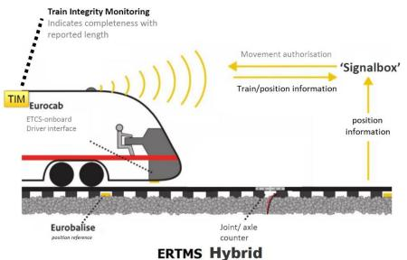
Figure 32: Hybrid Level 3 concept (Bartholomeus, Lecture: ERTMS Hybrid Level 3, 2020)
