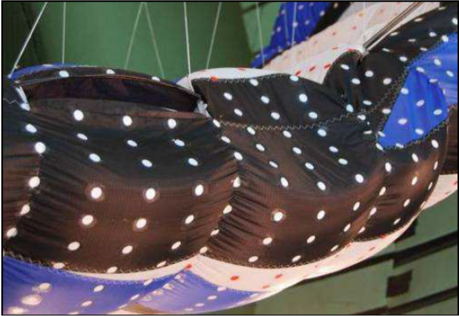
Figure 2.9: Ram-air kite in a wind tunnel experiment by de Wachter [23]. The white dots were used to compute the deformed shape of the parafoil for a CFD analysis. A striking detail are the dents located at the leading edge where the stagnation pressure compresses the membrane structure and the profile loses its curvature.
