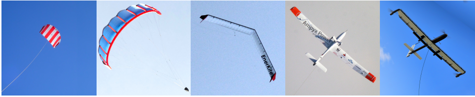
Figure 1.2: Soft, hybrid, and fixed-wing kite designs from various companies [12]. From left to right: SkySails Power, Kite Power, EnerKite, Ampyx Power, and TwingTec.
