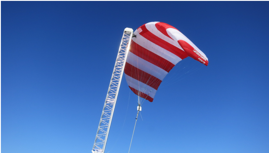
Figure 1.4: SkySails Power PN-14 system with inflated kite connected to mast.
