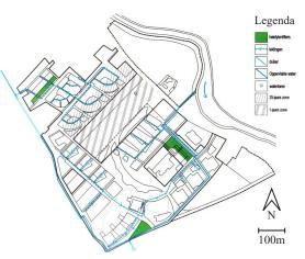
Figure 10. The greywater system of Lanxmeer with the helophyte filters (EVA-Lanxmeer, n.d.)
