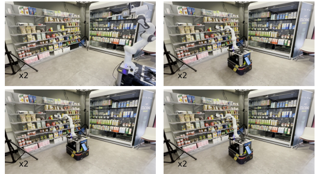
Fig. 7: Trajectory generation with optimization fabrics for mobile manipulator using visual servoing for product picking.
