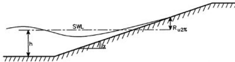
Figure 2.2: Wave run-up level  $R_u$  (Van der Meer and Janssen, 1994)
