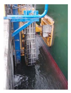
Figure 2.1 A MoorMaster<sup>™</sup> unit connected to a ship hull
