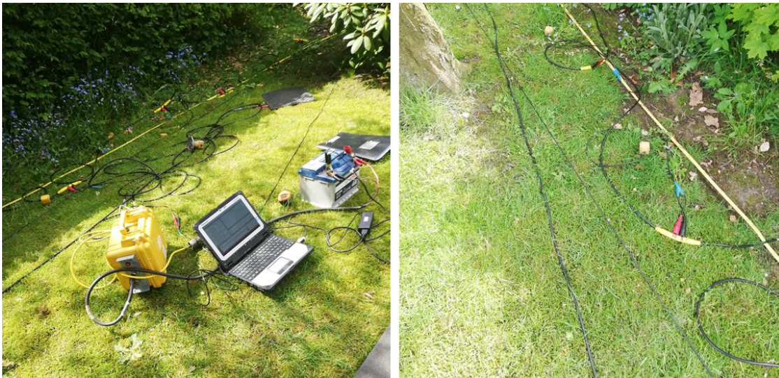
Figure 16 Setup of the measuring equipment (left) and Geophones inserted into the ground (right)
