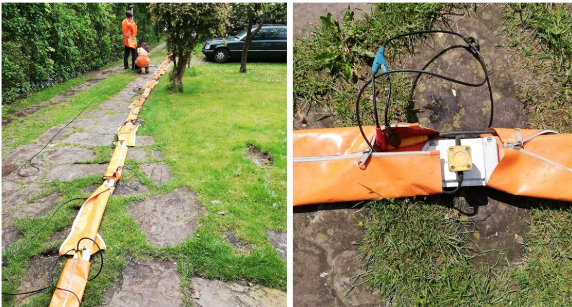
Figure 17 Streamer placement on sealed surface (left) connected single geophone (right)
