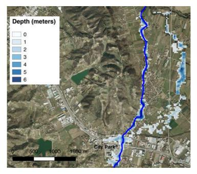
Figure 17: Flooded area for the *do nothing* alternative in the location of study.
