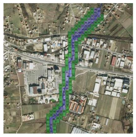
Figure 26: Ground elevation of the watershed of the Limuthi river in the City Park stretch.
