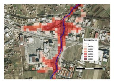
Figure 24: Target area to be protected from flooding.
