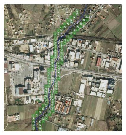
Figure 28: Determination of the type of retaining structure to be applied in every cross section of the Limuthi river, when passing through the City Park. '1' refers to the use of flood walls, in combination with dredging works in the river bed. '2' refers to the implementation of dikes, in combination of temporary structures (Slamdam) and dredging works in the river bed.
