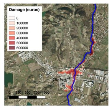
Figure 18: Damage (euros) produced in the area of study, given the flood event of design.
