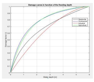
Figure 15: Normalized damage factor for Europe, in function of the flood depth, for industrial, commercial and agricultural areas.
