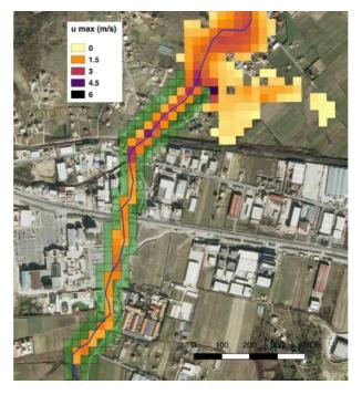
Figure 29: Maximum flow velocities in the analyzed stretch of the Limuthi river, during a 100-year return period flood event.
