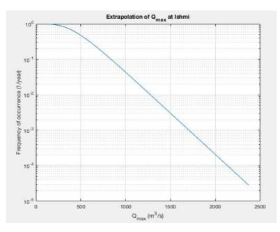
Figure 12: Frequency of occurrence  $(1/T_r)$  vs monthly maximum discharge (extrapolated function).
