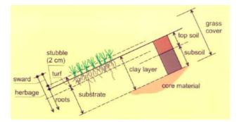
Figure 30: Composition and definitions of a grass on clay (Jonkman et al. (2018)).
