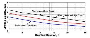
Figure 31: Relationship between the flow velocity, the duration of the overflow and the quality of the grass.
