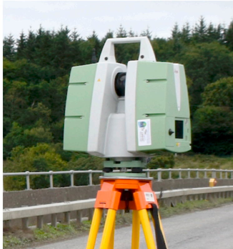
Figure 12. P20 laser scanner.
