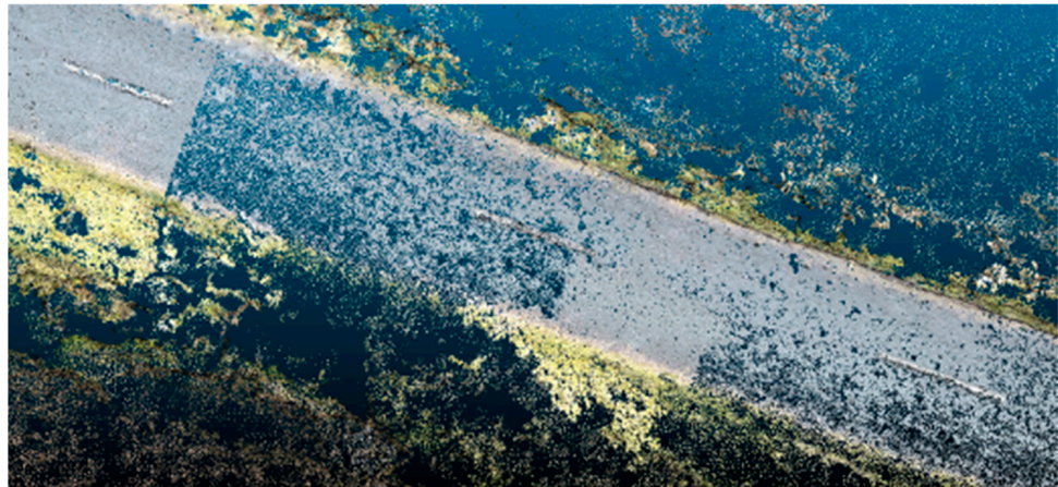
Figure 2. Incomplete dataset in SfM roadway point cloud.
