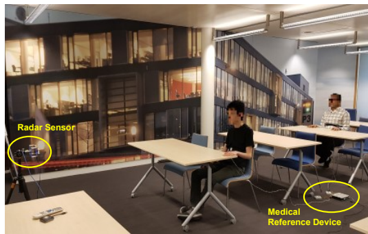
Fig. 5: Experimental environment mimicking an educational class setting. In the figure, the two volunteers are respectively at about 2 m and about 5 m distance from the radar. A medical reference device was used to measure the heartbeat (through PPG sensors with finger transducers) and respiration (through belt sensors) of the volunteers.
