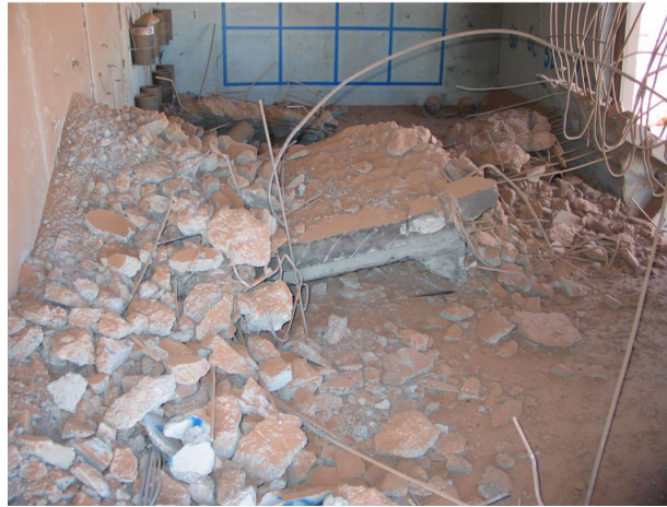
Figure 1: Heavy spalling as encountered in a field experiment by TNO. The blast came from the right side of the figure. (Wees et al., 2007)
