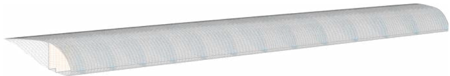
Example of a quadrilateral mesh of the wing tip section generated from the MegAWES [2] reference kite (colorized for illustrative purposes).
