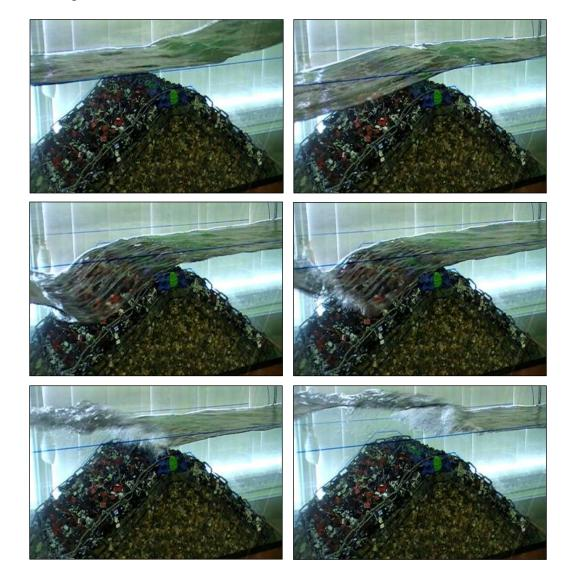
Figure 6.2 Current in seaward direction over breakwater crest for test series BI 2
