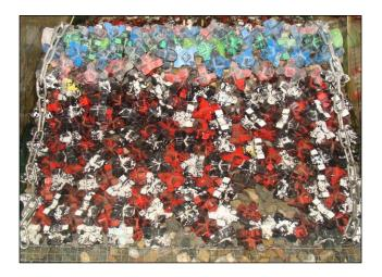
In test AII\_2 the Xbases displaced a significant distance resulting in excessive settlements in the armour layer of the leeward slope. The test is executed again (test AII\_2\_1) with fixed Xbases in lateral direction (see Figure 5.7).
