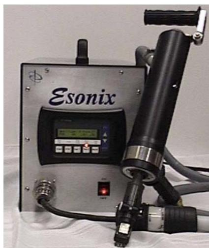
*Fig. 7-1: UIT generator and peening tool [30].*
