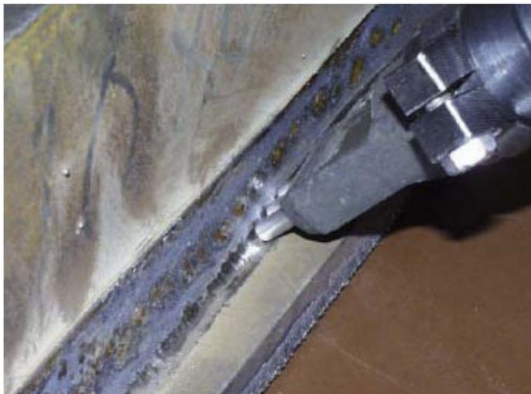
*Fig. 2-4: Application of UIT with multiple indenters at the toe of a weld [34].*
