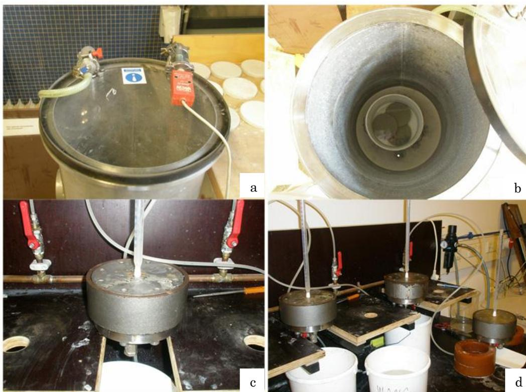
*Figure 4.1. Setup of the experiment. (a). Vacuum machine. (b). Specimens in the Vacuum machine. (c). Set-up cell for the test. (d). Three parallel samples.*
