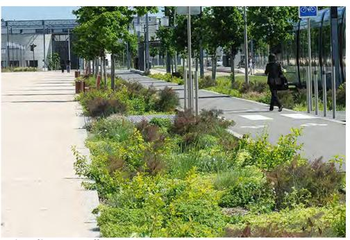
Swales to filter storm runoff
