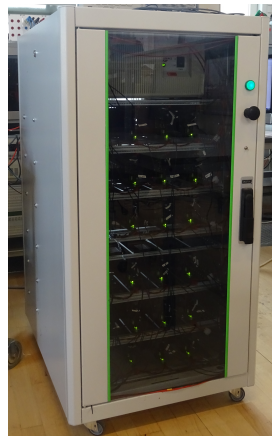
Figure 7. Laboratory prototype of the MMC STATCOM.
