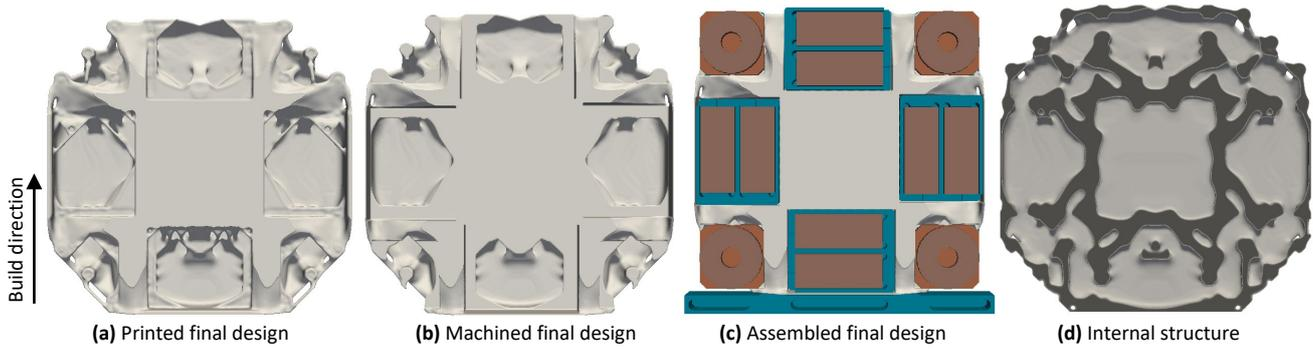
**Figure 2.** The optimized design at different process steps: (a) the design after additive manufacturing, (b) the design after machining, (c) the final assembled design, and (d) a crosssection showing internal structures. The arrow indicates the build direction.
