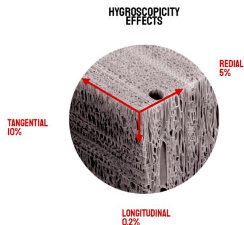
Figure 110 Fiber direction shrinkage ratio taken from PhD candidate Max Salzberger.
