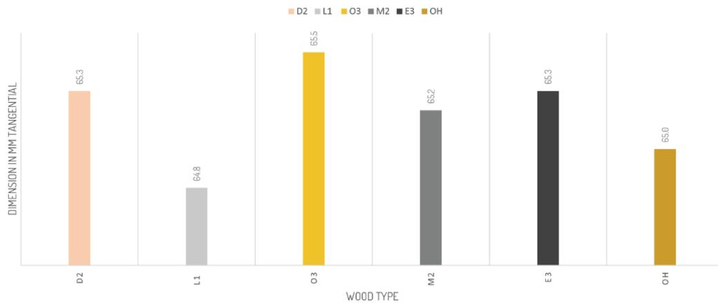
Figure 106 Final dimensional change in tangential fiber direction after 30 days
