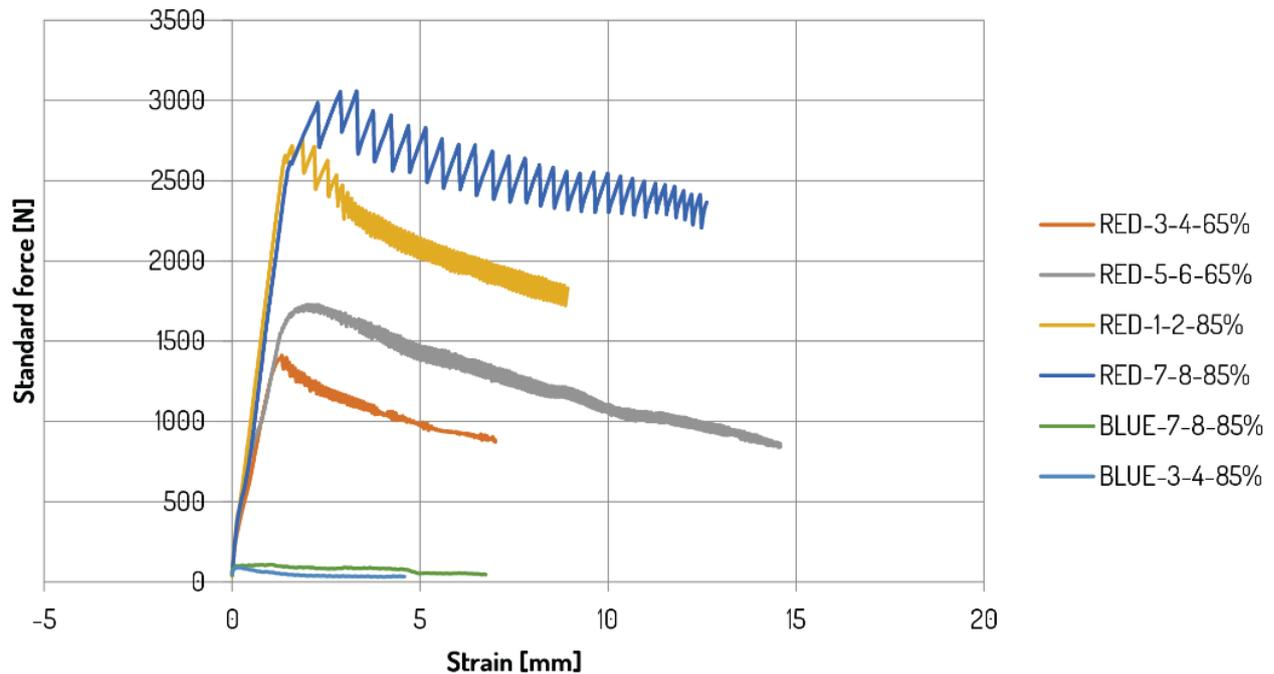
Figure 118 Tensile Test Result of moisture induce Cross Half Lap joints
