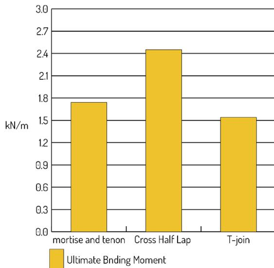
Figure 116 Ultimate Bending Moment Capacity
