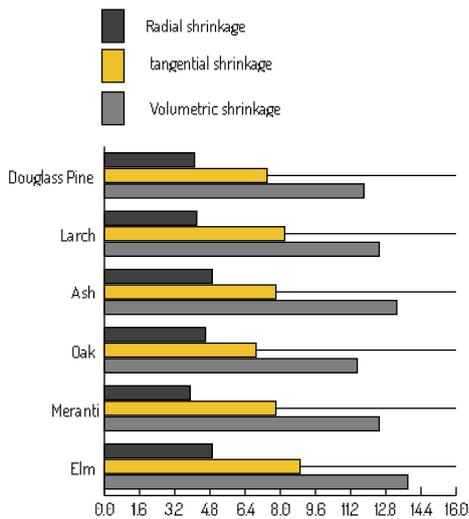
Figure 107. Tangential, radial and longitudinal Shrinkage of several wood species
