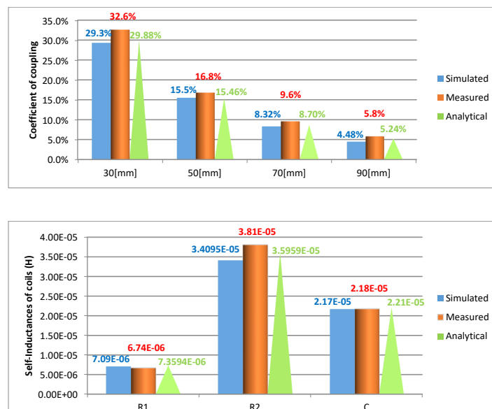
Figure 10. Coupling coefficient and self-inductances of air-cored charge pads of various shapes. The coupling is measured at various z-gaps at the best aligned point. The parameters of the coils are as presented in Table 1.
