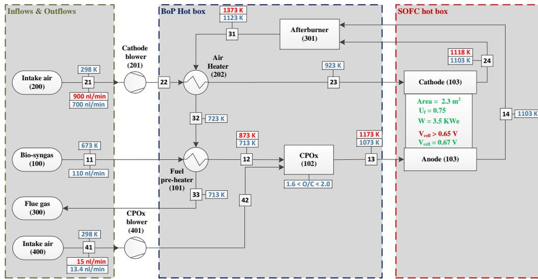
**Figure 3.** Limiting operation and preliminary design parameters of the SOFC system. Red parameters: maximum volume flows and temperatures; blue parameters: preliminary design parameters. BoP: balance-of-plant; CPOx: catalytic partial oxidation unit.
