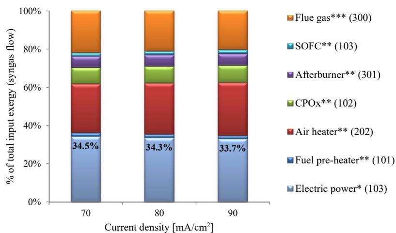
**Figure 9.** Exergy distribution into the various types of exergy produced in the system. \* Net electric power; \*\* Exergy destruction per component; \*\*\* Exergy loss carried by the flue gas.
