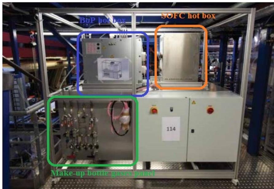
**Figure 2.** The SOFC 3.5 kW<sub>e</sub> system at TU Delft with description of the various parts. The air blowers are located behind the make-up bottle gases panel.
