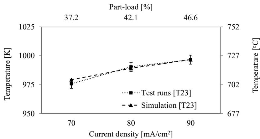
**Figure 7.** Comparison of simulated results with those acquired in the test runs. Cathode air from air heater ( $T_{23}$ ).
