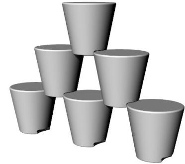
▲ Figure 4.9 CAD model examining the feasibility of stacking.
