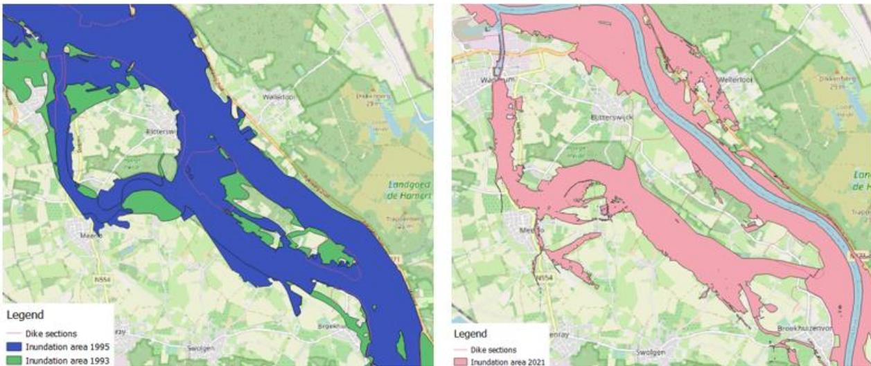
**Figure 62: Inundation areas of Ooijen and Wanssum in 1993 and 1995 with the future dike sections (right side) and Inundation area of 2021 with their current dike sections (left side)**
