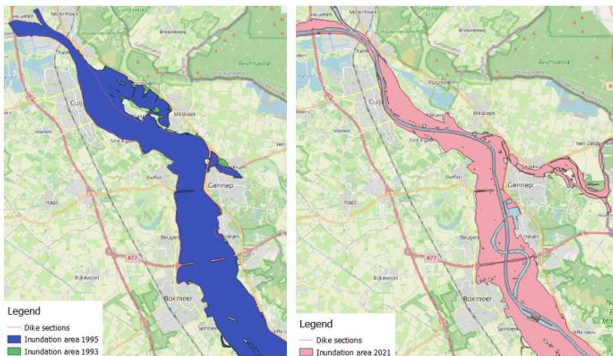
**Figure 64: Inundation areas of Genneep and Boxmeer in 1993 and 1995 with the future dike sections (right side) and Inundation area of 2021 with their current dike sections (left side)**
