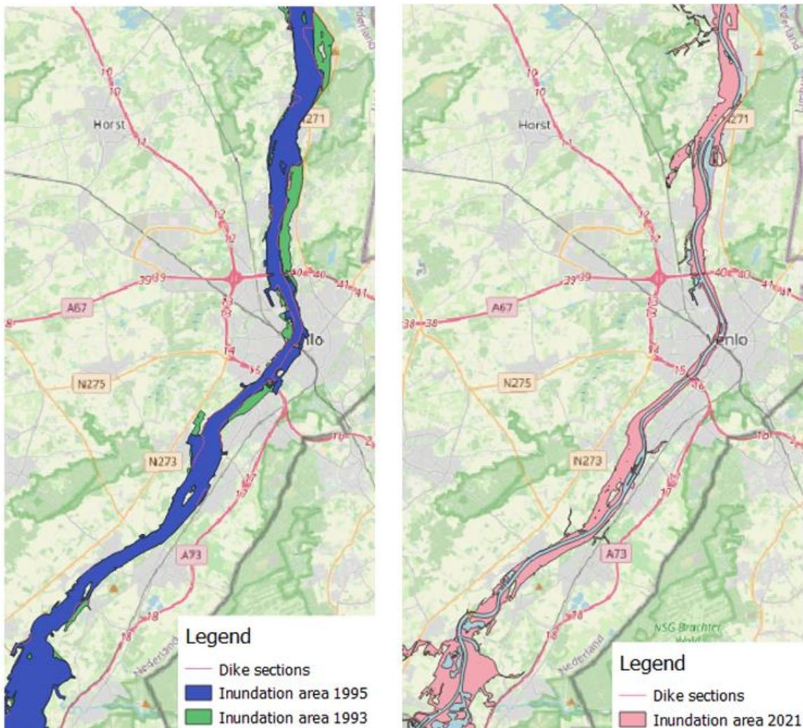
**Figure 59: Inundation areas of the Peelhorstmaas in 1993 and 1995 with the future dike sections (right side) and inundation area of 2021 with their current dike sections (left side)**
