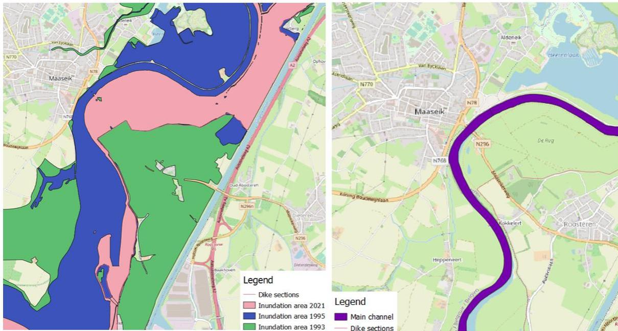
Figure 55: A map of Maaseik and Roosteren with the inundation areas of the different floods (left side) and with the dike sections and the main channel (right side)
