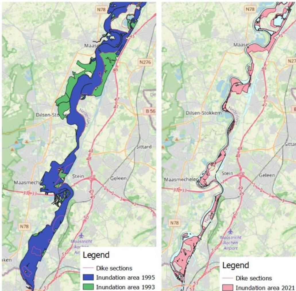
Figure 48: Inundation area of the Grensmaas in 1993 and 1995 with the future dike sections (right side) and Inundation area of 2021 with their current dike sections (left side)
