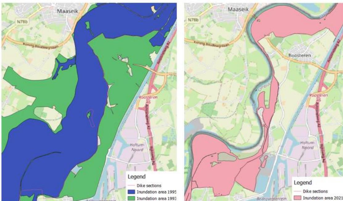
Figure 54: Inundation areas of Ilkhoven, Visserweert and Roosteren in 1993 and 1995 with the future dike sections (right side) and Inundation area of 2021 with their current dike sections (left side)
