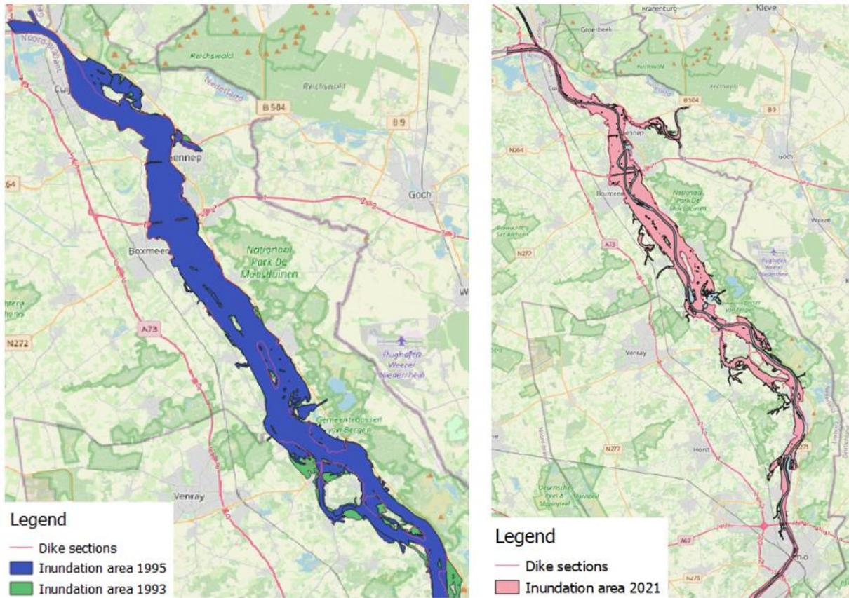
Figure 61: Inundation areas of the Venloslenkmaas in 1993 and 1995 with the future dike sections (right side) and inundation area of 2021 with their current dike sections (left side)
