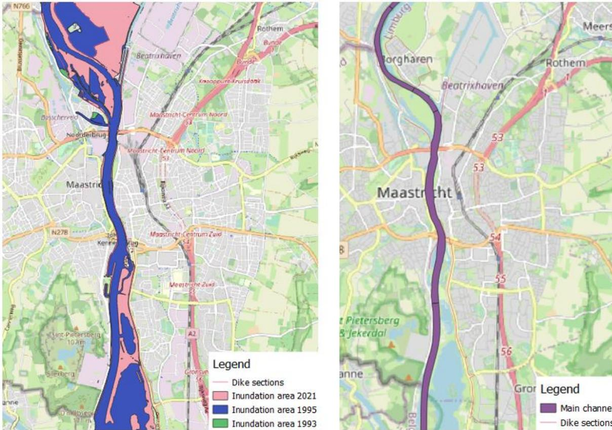
**Figure 11: A map of Maastricht with the inundation areas of the different floods (left side) and with the dike sections and the main channel (right side)**
