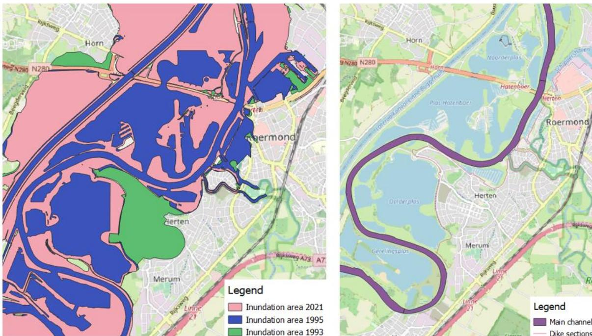
**Figure 58: a map of Roermond with the inundation areas of the different floods (left side) and with the dike sections and the main channel (right side)**
