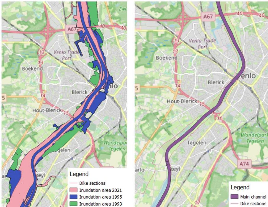
**Figure 20: A map of Venlo with the inundation areas of the different floods (left side) and with the dike sections and the main channel (right side)**
