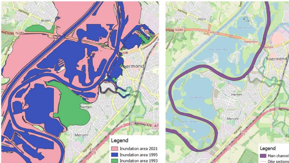
**Figure 17: A map of Roermond with the inundation areas of the different floods (left side) and with the dike sections and the main channel (right side)**
