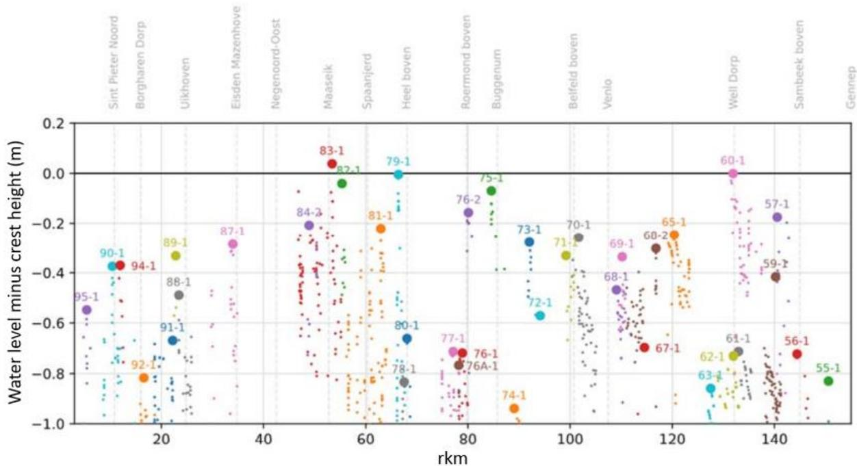
**Figure 44: Differences between crest height derived from AHN3 and modeled water levels for all dike sections along the Meuse between the Dutch border and Gennepep (ENW, 2021)**
