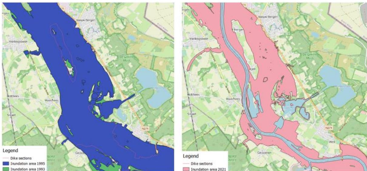
**Figure 63: Inundation areas of Elsteren and Aijen in 1993 and 1995 with the future dike sections (right side) and Inundation area of 2021 with their current dike sections (left side)**
