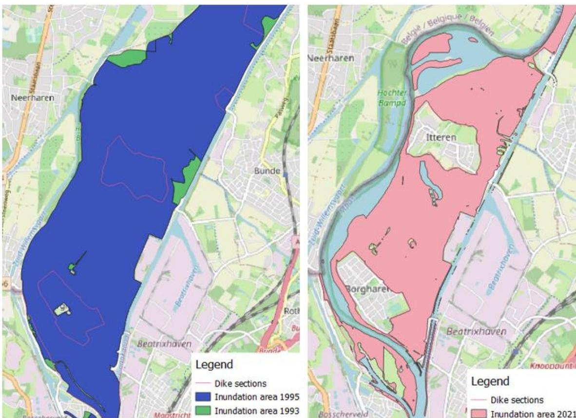
Figure 50: Inundation areas of Borgharen and Itteren in 1993 and 1995 with the future dike sections (right side) and Inundation area of 2021 with their current dike sections (left side)
