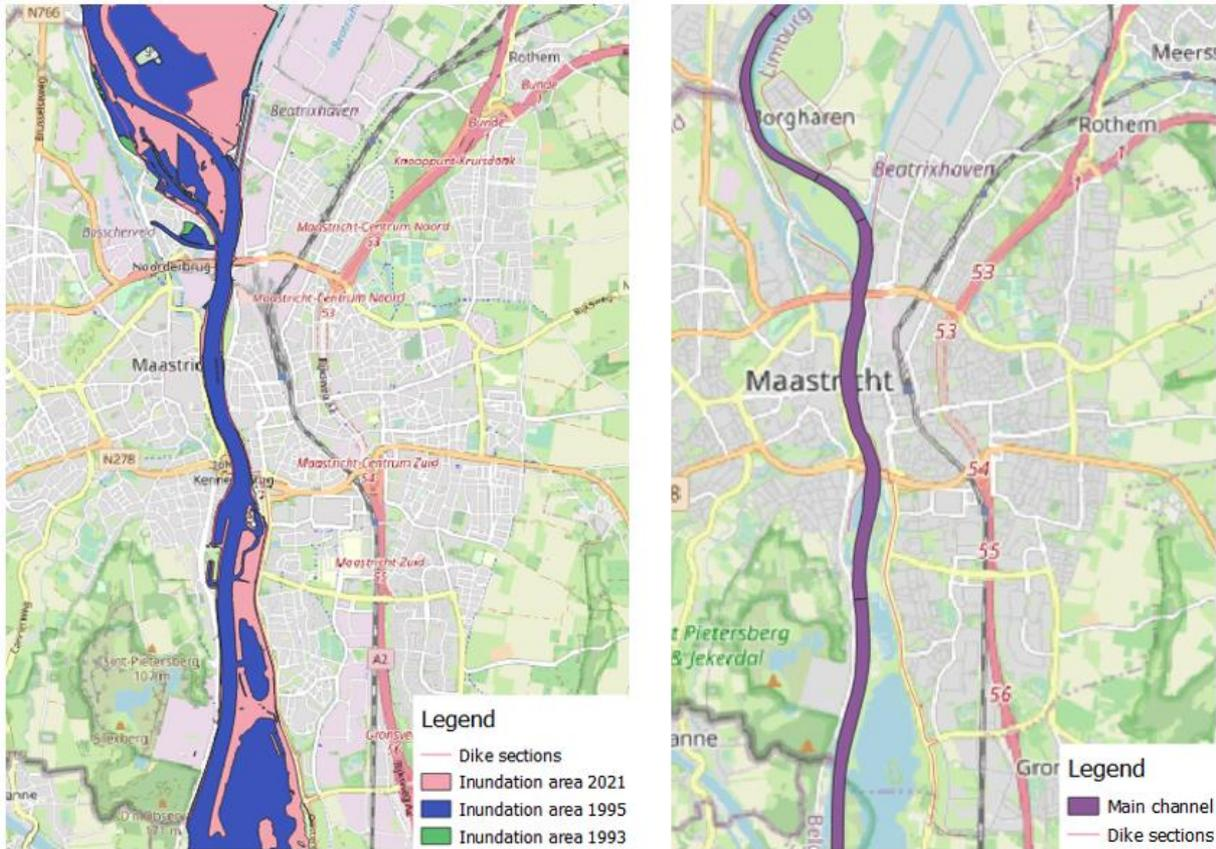
**Figure 49: A map of Maastricht with the inundation areas of the different floods (left side) and with the dike sections and the main channel (right side)**
