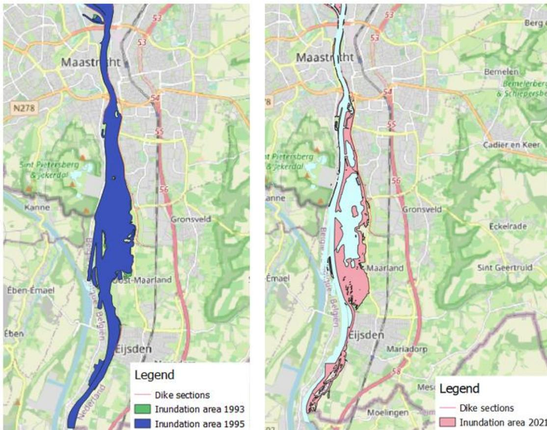
Figure 47: Inundation area of the Bovenmaas in 1993 and 1995 with the future dike sections (right side) and Inundation area of 2021 with their current dike sections (left side)
