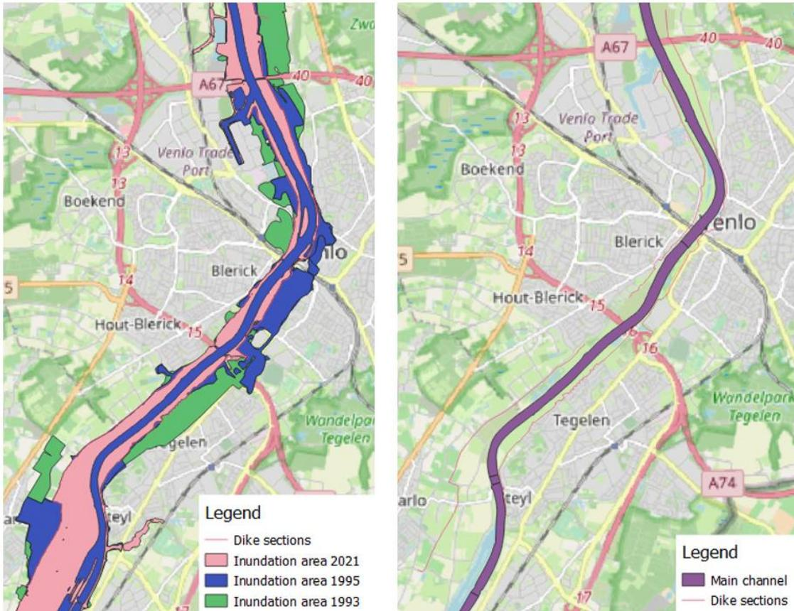
Figure 60: A map of Venlo with the inundation areas of the different floods (left side) and with the dike sections and the main channel (right side)
