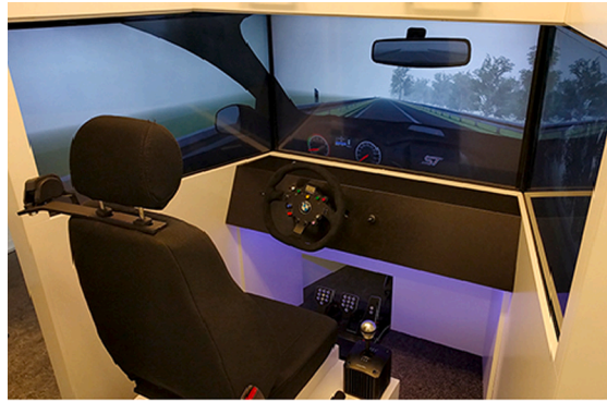
Fig. 2. The fixed-based driving simulator.
