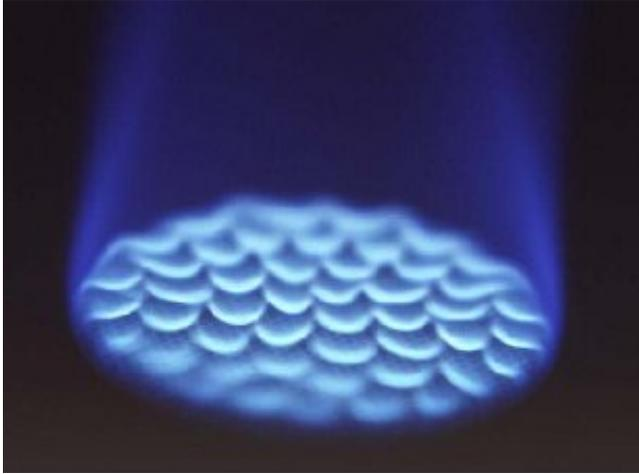
Figure 32: Picture of a real flame with a cellular structure (from [www1.gifu-u.ac.jp](http://www1.gifu-u.ac.jp)).
