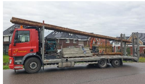
FIGURE 61 TIMBER PILES (SCHIPPER, 2021)
