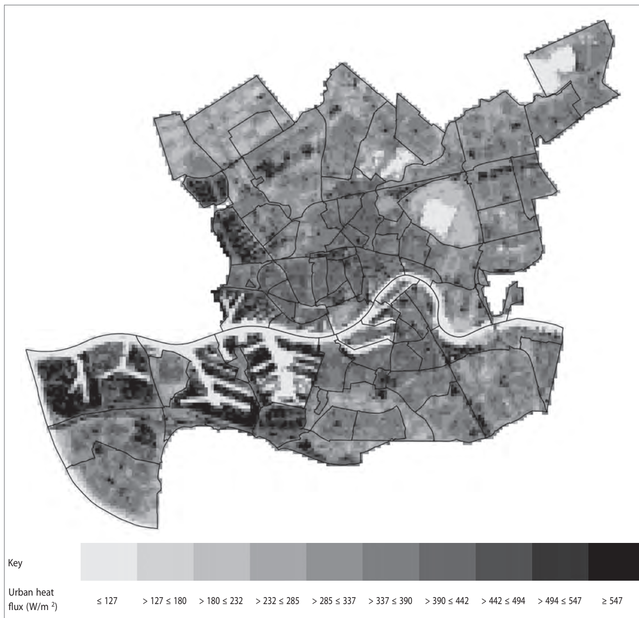
Figure 4: The sum of the sensible and storage heat fluxes, 16 July 2006 (author: Frank van der Hoeven).
