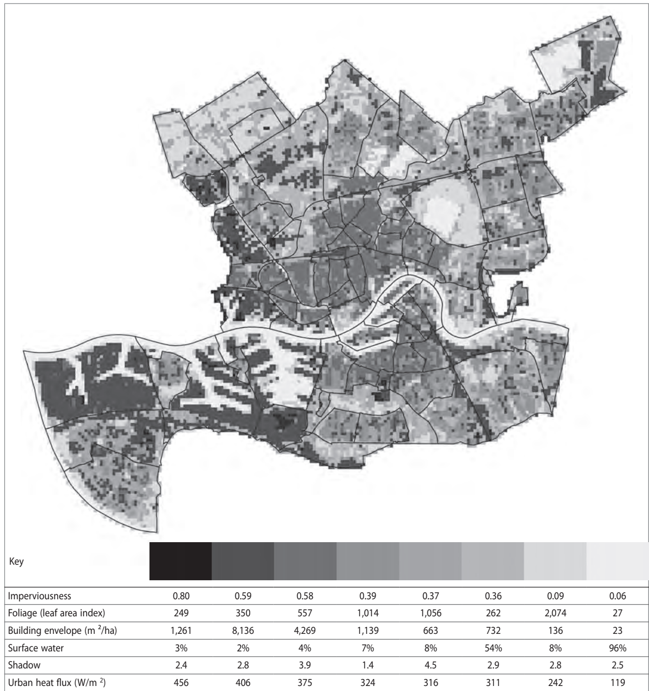
Figure 8: Spatial heat map: the spatial pattern of land use and urban form that contributes in a greater or lesser degree to the urban heat island in the city of Rotterdam (source: van der Hoeven & Wandl, 2015c).
