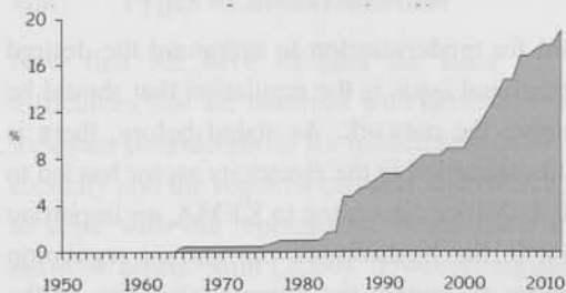
Figure 3 Planned increase of interconnections in the EU in % of installed generation capacity
