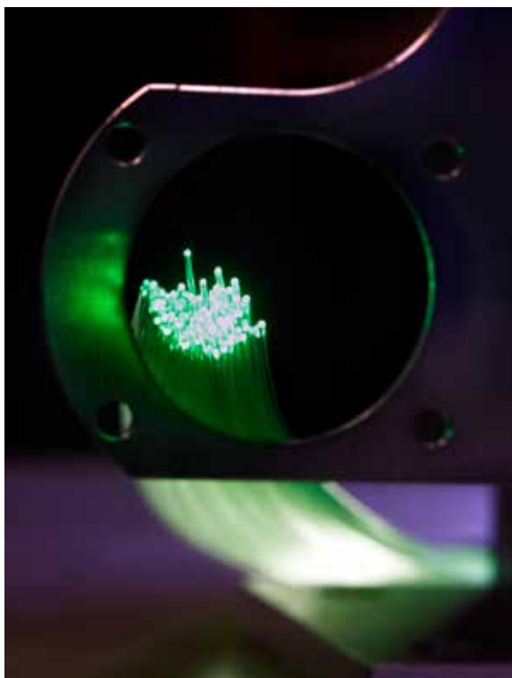
The sample is surrounded by a semi-circle containing 1,408 detectors.
