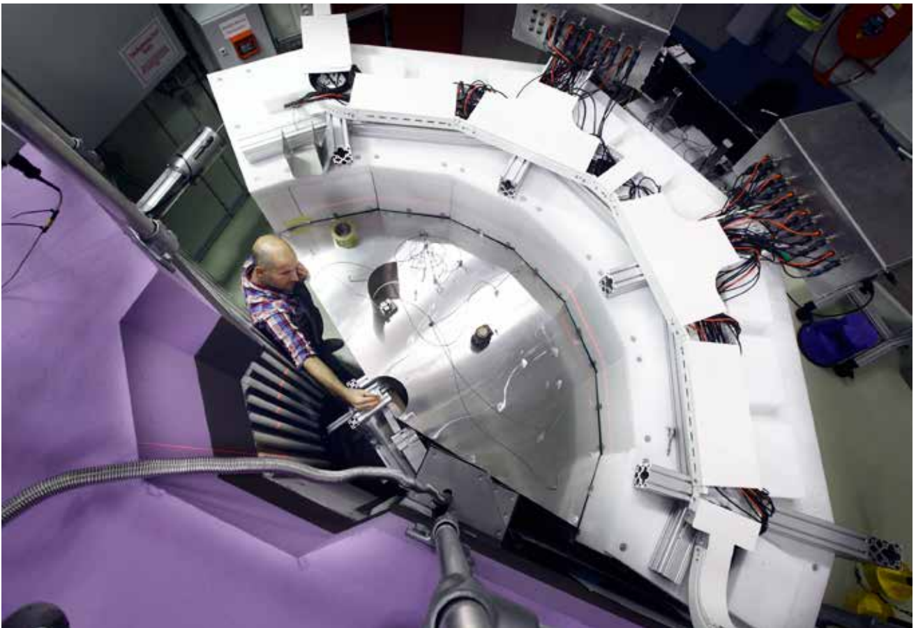
Lambert van Eijk places a sample in the centre of the diffractometer (right).
