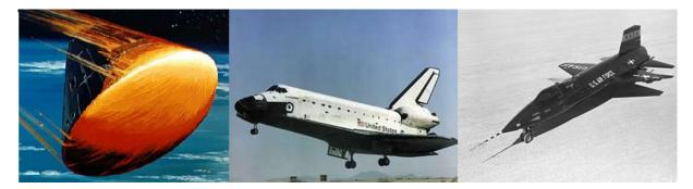
Figure 7: Types of Hypersonic vehicles; Left: Re-entry Apollo capsule (NREV) [113], Center: Space Shuttle (WREV) [47], Right: X-15 (CAV) [90].
