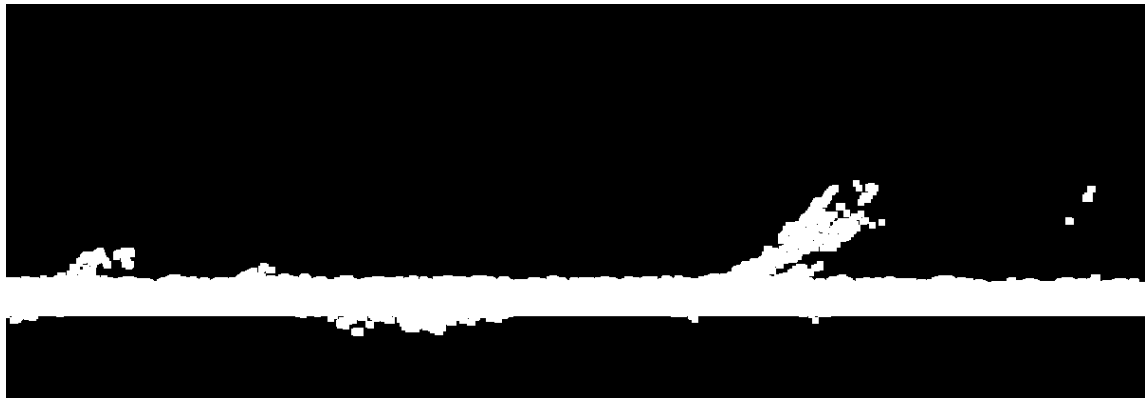
Figure 9: Erosion followed with dilation is the opening operator. High outliers are all removed and much of the low outliers as well. Even large part of the cluster noise is removed.
