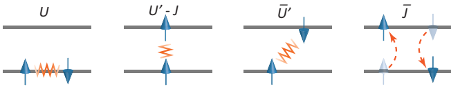
FIG. 3. On-site interactions within one quantum dot: Hubbard U , interorbital Hubbard U' (and its spin-antiparallel form \bar{U}' ), and Hund's exchange J (and its spin-antiparallel form \bar{J} ).
