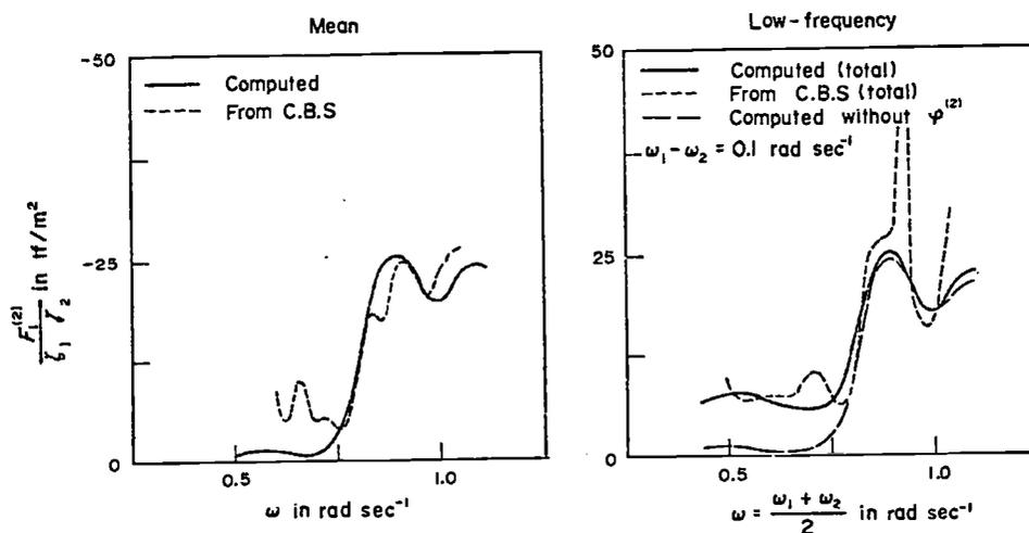
FIG. 8. Comparison of mean and low frequency surge drifting forces.
