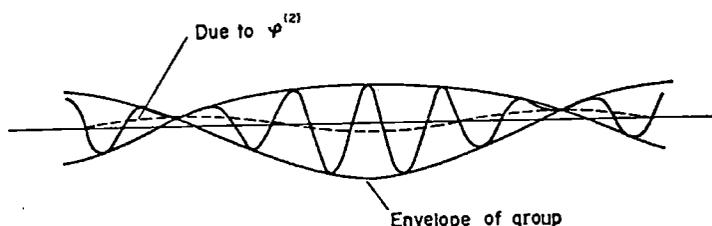
FIG. 9. Wave due to second order potential in a wave group.
