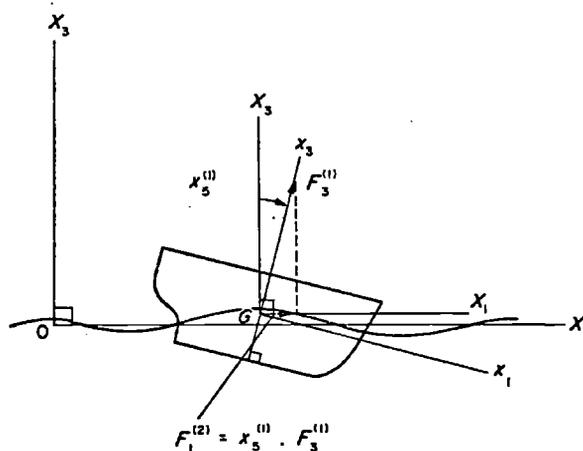
FIG. 1. Contribution of pitch angle and heave force to second order surge drifting force.
