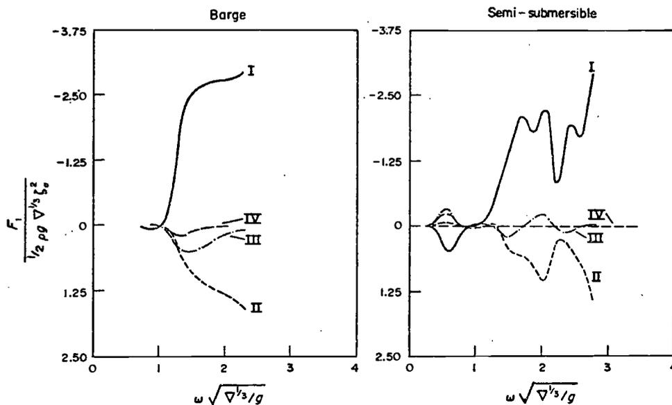
FIG. 4. Components of the computed mean surge drifting force.
