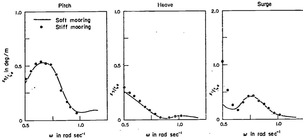
FIG. 7. First order motions of the semi-submersible in head waves.
