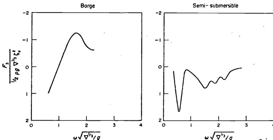
FIG. 5. Computed mean heave drifting force.
