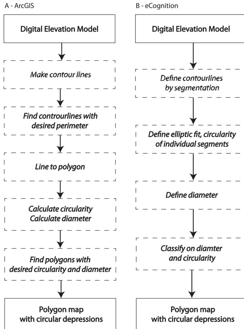
**Figure 3.3:** Flowchart depression recognition using (A) ArcGIS or (B) eCognition
