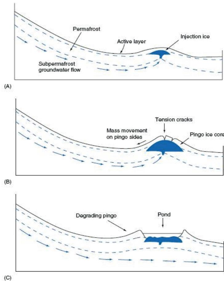
**Figure 1.2: Formation of hydraulic system pingos (Ballantyne & Harris, 1994)**
